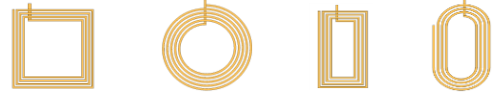
Fig. 1: The four micro coil types of geometries studied (circular, square 1000 \times 1000 \mu\text{m}^2 , rectangular and ellipsoidal 1000 \times 500 \mu\text{m}^2 ).
